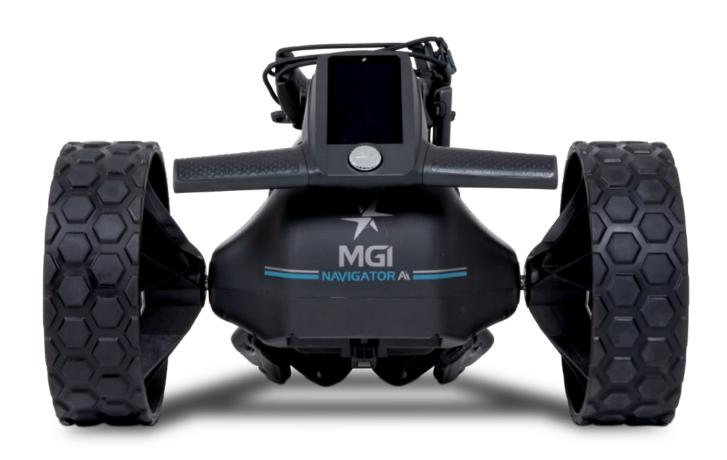
Press the black release button on the wheel hub. Place the wheel onto the axle. You will need to match up the inner female groove on the axle and the male of the wheel. See Section 3.3 for Rear Wheels Position.
